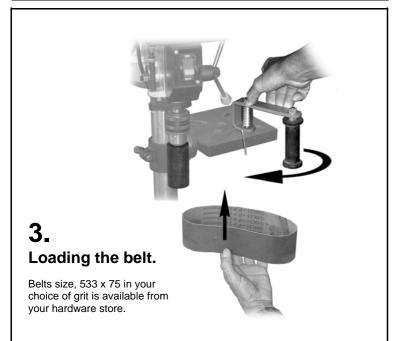
**Belt Tension:** Rotate the drill table away from the drive drum until a suitable tension is achieved. **NOTE:** insufficient belt tension will cause the belt to be unstable in its position on the drums during sanding.
