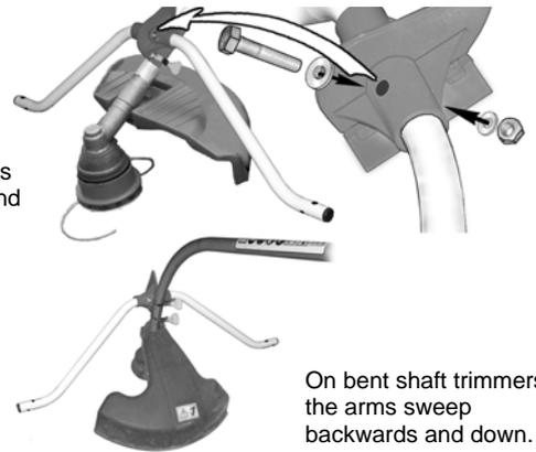
On bent shaft trimmers the arms sweep backwards and down.
