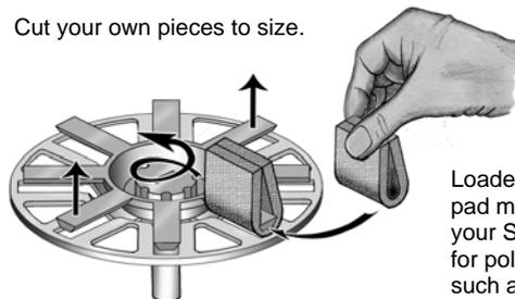
Loaded with scouring pad material you can use your SPIDER SANDER® for polishing materials such as sheet metals etc.
