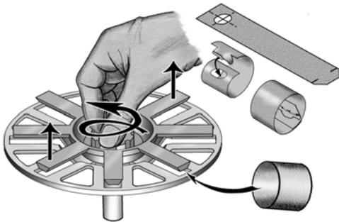
1. Loosen the locking screw until the fingers lift clear of the sander body.
